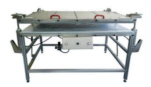
STK Lab impregnated paper requires strong and even pressure to press STK Lab paper against analyzed evidence without moving. These press devices are designed to ease work in the lab and to give reproductible results.
