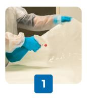
Cut a piece of STK Lab. Using a sprayer, **saturate STK Lab absorbing side** with demineralized water
